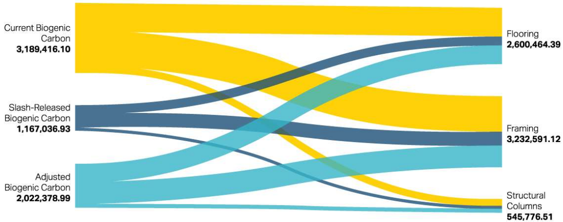
Figure 8. The differences between the current biogenic carbon (in kg CO 2 e), the slash-released carbon (in kg CO 2 e), and the adjusted biogenic carbon (in kg CO 2 e) for the three building components considered in the study in the A1 scope
